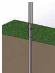
2. Put the post into the ground screw.
