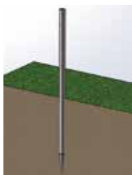
1. Drive the ground screw into the soil.
