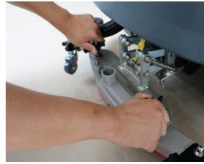
逆时针拧下固定螺母 Unscrew the fixing nut counterclockwise
