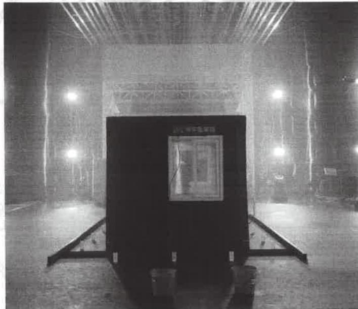
Test-in-process (rainfall intensity: 60mm/h)
