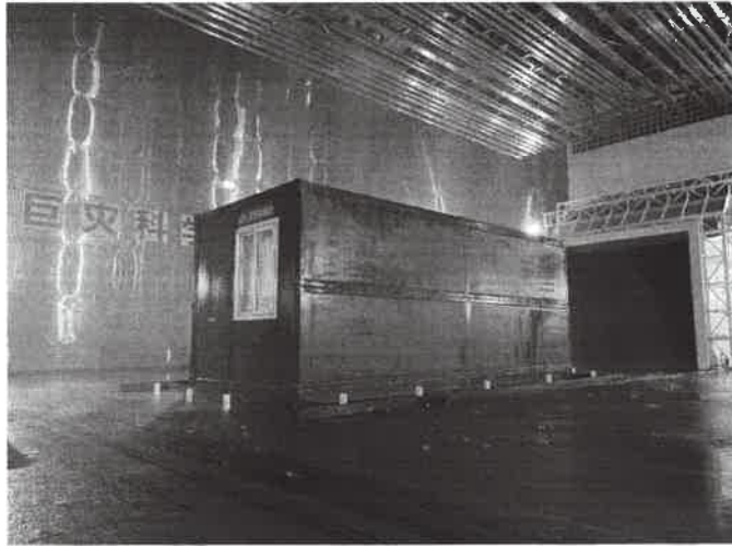
Test-in-process (rainfall intensity: 30mm/h)
