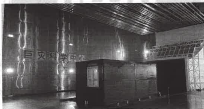
Test-in-process (rainfall intensity: 27mm/h, wind speed: 10m/s)
