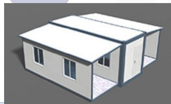
Setp 3 Open walls
